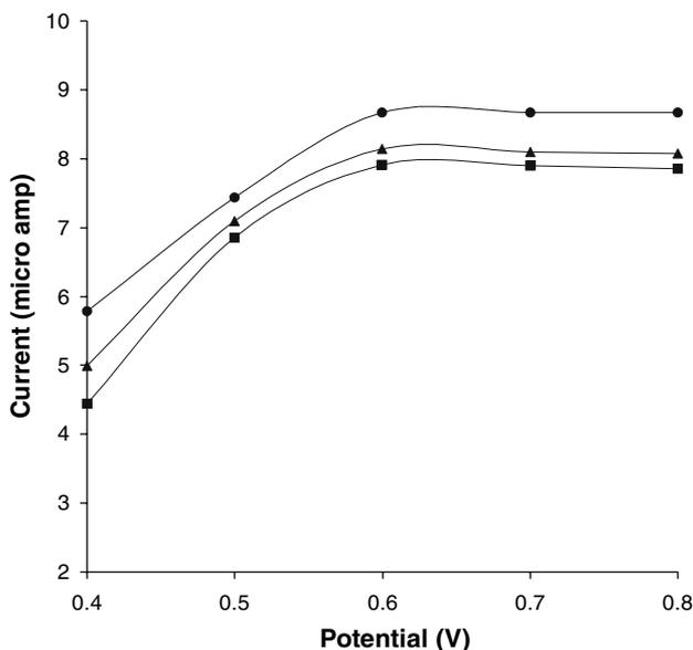
**Fig. 6** Current–potential curves for the GOD electrode of PA (■), POA (●) and PA-co-POA (▲), in 0.1 M acetate buffer, 20 mM glucose and pH 5.5
