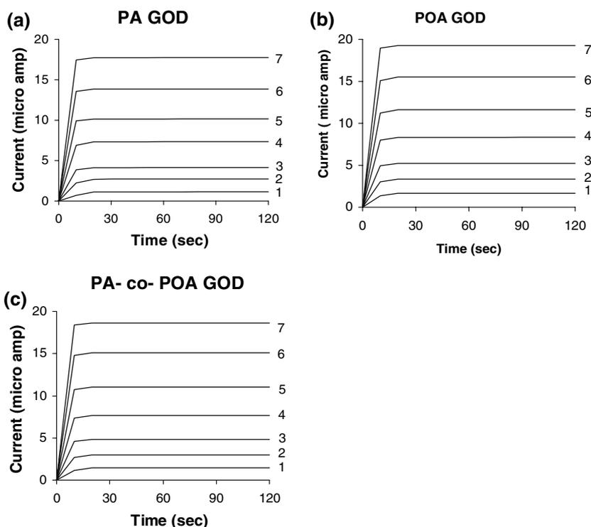
**Fig. 2** Current–time curves for the GOD electrode of (a) PA, (b) POA and (c) PA-co-POA at 0.60 V Glucose solution (1) 1 mM, (2) 5 mM, (3) 10 mM, (4) 20 mM, (5) 30 mM, (6) 40 mM, (7) 50 mM, in 0.1 M acetate buffer, pH 5.5
