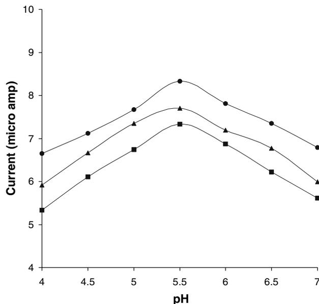
**Fig. 7** Effect of pH on the GOD electrode response of PA (■), POA (●) and PA-co-POA (▲). Steady state currents measured at 0.60 V in 20 mM glucose solution in 0.1 M phosphate buffer
