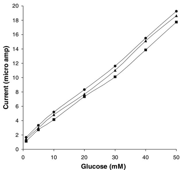
**Fig. 3** The relationship between response current and glucose concentration for the GOD electrode of PA (■), POA (●) and PA-co-POA (▲), in 0.1 M phosphate buffer, pH 5.5
