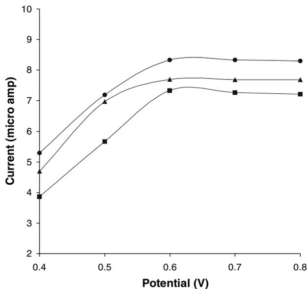
**Fig. 5** Current–potential curves for the GOD electrode of PA (■), POA (●) and PA-co-POA (▲), in 0.1 M phosphate buffer, 20 mM glucose and pH 5.5
