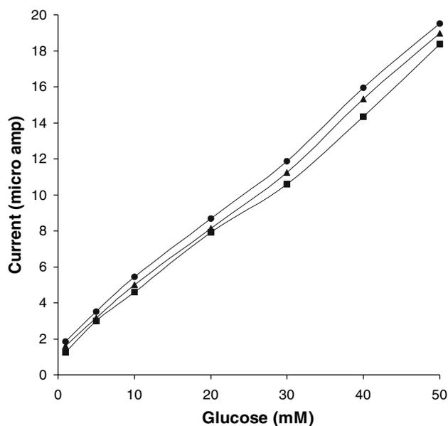
**Fig. 4** The relationship between response current and glucose concentration for the GOD electrode of PA (■), POA (●) and PA-co-POA (▲), in 0.1 M acetate buffer, pH 5.5
