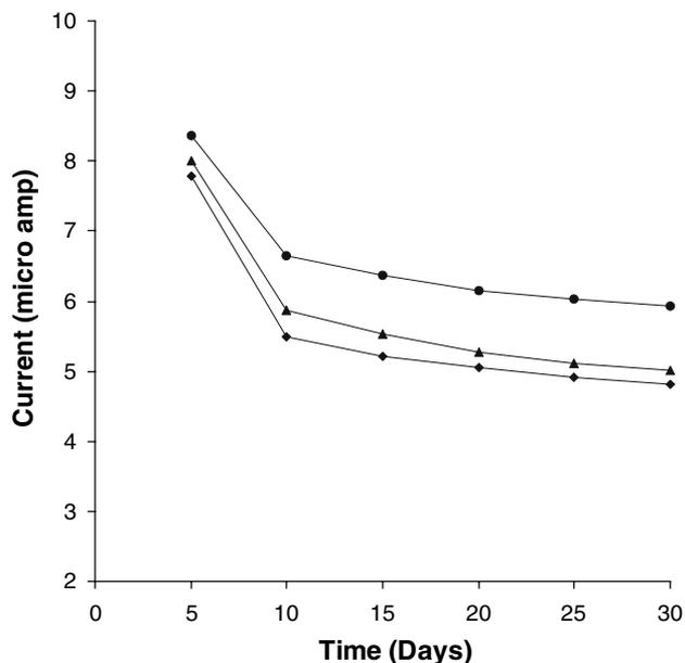
**Fig. 10** Stability of the PA (■), POA (●) and PA-co-POA (▲) GOD electrode on storage in 0.1 M acetate buffer, 0.6 V and pH 5.5 at room temperature
