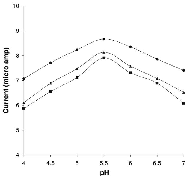
**Fig. 8** Effect of pH on the GOD electrode response of PA (■), POA (●) and PA-co-POA (▲). Steady state currents measured at 0.60 V in 20 mM glucose solution in 0.1 M acetate buffer
