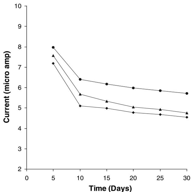
**Fig. 9** Stability of the PA (■), POA (●) and PA-co-POA (▲) GOD electrode on storage in 0.1 M phosphate buffer, 0.6 V and pH 5.5 at room temperature
